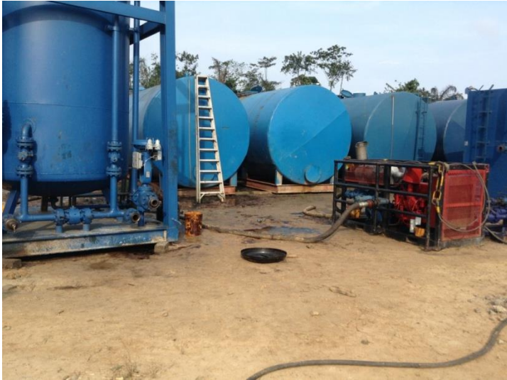
10-11: Recovery pump (Pic10) and Recovered Crude sighted in Recovery containers (Pic11)
